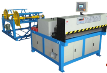
DUCT AUTOMATIC LINE III
